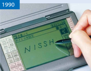
Developed resistive-type touch sensors
